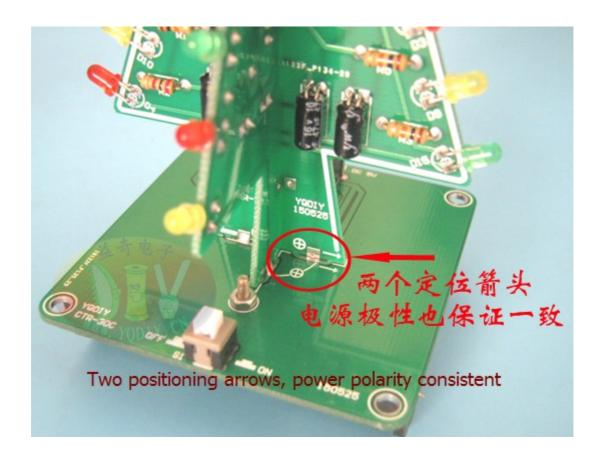
16. Welding the top LED (with direction)
