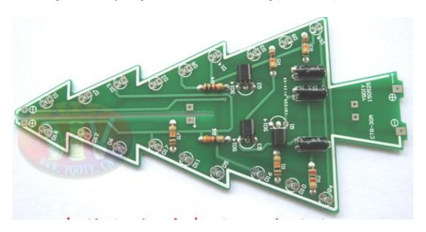
5. Welding red LED (with direction)), the red LED numbered D1  $\sim$  D6.
