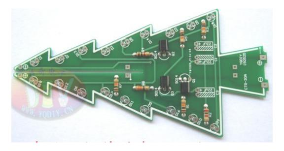
4. Welding three electrolytic capacitors, use horizontal mounting (with direction)
