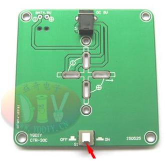
13. A board and B board combination (with direction, the two plates are positioned like the arrow below), after two positioning arrows are aligned, use a soldering iron to put the two board together.
