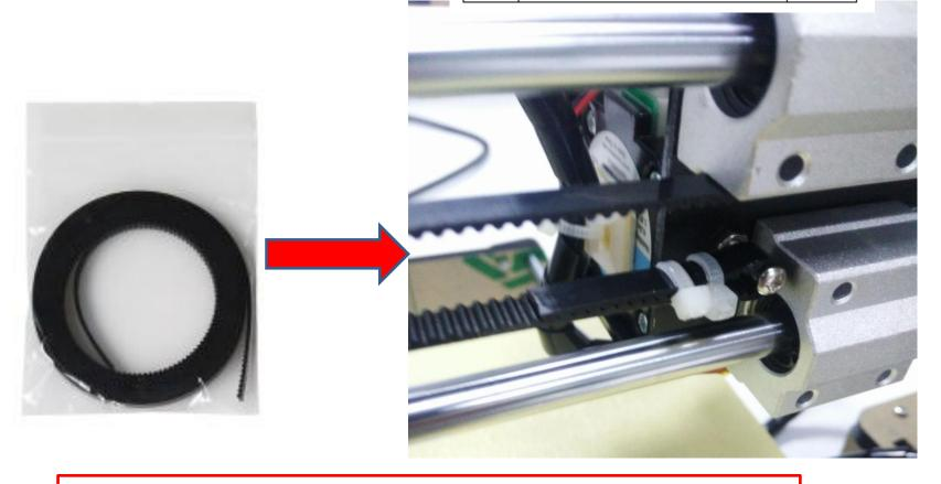
Attention: Belt is for X,Y axis transmitting. The length of belt is 1.5m in total. Normally there'll be 10-20cm left after installation.
