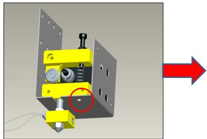
Loose M4\*6 screws first, then separate extruder from L black aluminum parts, remember to keep the screws.
