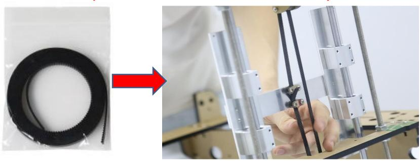
Attention: Belt is for X&Y axis transmitting .Cut the length you need to each transmission shaft. The belt is 1.5m in total and 10-20cm left after installation.
