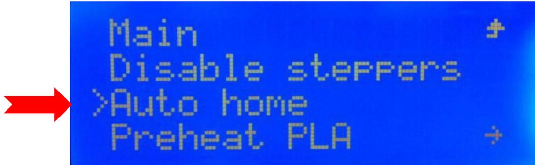
Note: Select "AUTO HOME" instruction, the axes will move to the zero position (bottom left corner), after hit limit switch stops. Make sure the Z-axis limit switch is installed correctly (see assembly section detail view) or nozzle will spray to the platform while executing this command.
